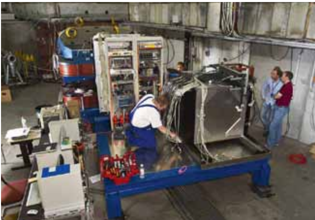
Figure 6.5 Test setup for the CLIC W-HCAL. Left image: CERN Bulletin . Right image: CERN LCD.
