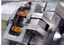
(a) Saclay/DESY tuner mounted on the cavity jacket
