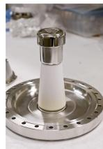
High voltage processing in the presence of inert gas (He and Kr) was demonstrated to significantly improve the performance of stainless steel and niobium cathode electrodes, eliminating field emission (< 10 pA) at voltages to 225 kV and field strengths > 18 MV/m [217] (see Fig. 4.6).
