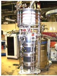
(b) The split quadrupole mounted on the insert of the cryostat.
