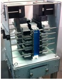
(b) Permanent magnet for beam focusing in the DRFS klystron.
