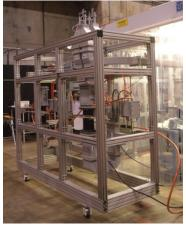
(a) A two-feed unit of PDS1, incorporating a VTO and H-hybrid, installed on a cryomodule at NML.
