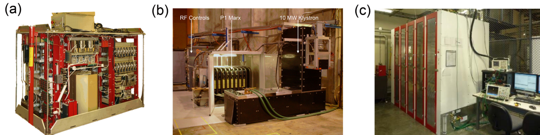
Figure 3.28. (a) DTI Marx modulator, (b) SLAC P1 Marx modulator and (c) SLAC P2 Marx.
