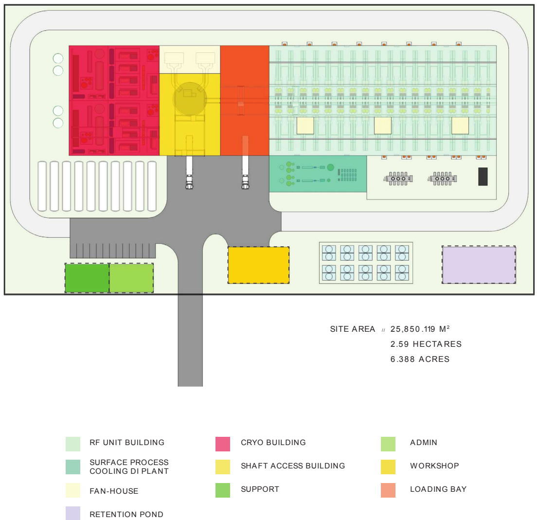
Figure 11.31. Typical KCS surface facility layout
