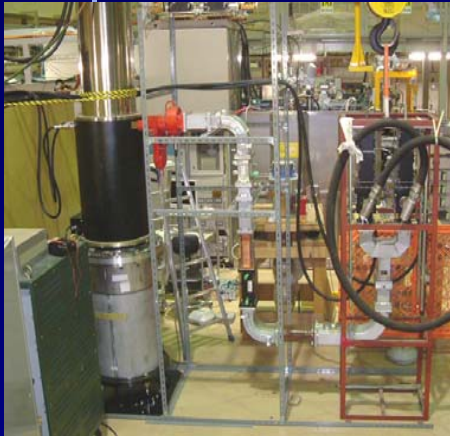
TH2104A old klystron short pulse test.
