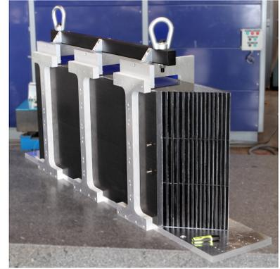
inserted into the alveoli of the mechanical structure. The insertion process has been successfully implemented for the physics prototype with short layers and has in addition been demonstrated with layers of up to 1.3 m length for a mechanical demonstrator of the technological prototype. In case of the ScECAL one side of the tungsten board will be equipped with scintillating strips for the  $x$  direction and the other side with strips for the  $y$  direction.
